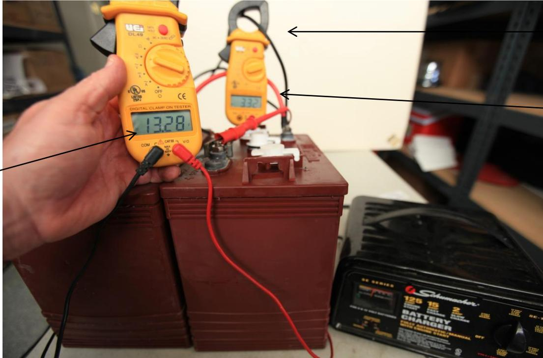
We have clamped over the wire and are now reading DC amps. The rate of charge in amps is 3.32. When batteries are low in charge the charger puts out a higher amount of amps. As the battery voltage increases the amperage goes down to below 1 amp when fully charged. You should see at least 15 amps going into the batteries when they are low in charge.
