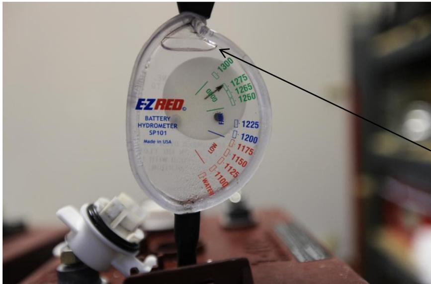
This is the proper level. Remember to shake the hydrometer a little to get any air bubbles out.
